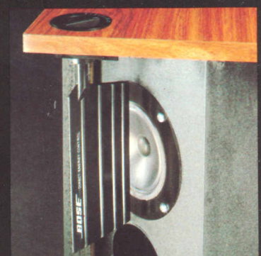
The Direct Energy Control adjusts the spatial properties of the 301 speaker by controlling the radiation pattern of the side-angled tweeter.
